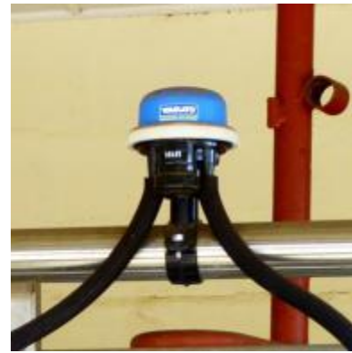
An automatic pulsator to 'rest' the cows while milking. It is mounted on the vacuum line and serves two cows.
