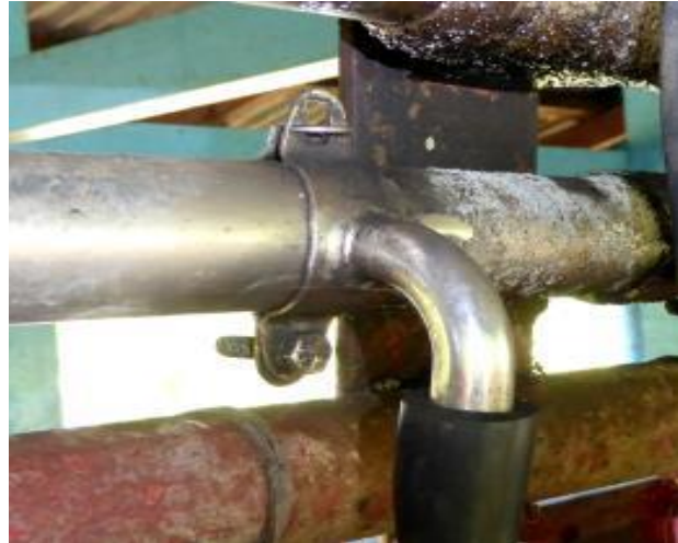
Connection to the vacuum system with clamp-on fitting plus snap clamp as shut-off valve.
